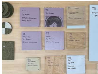
PET felt and plywood for pinning up.
