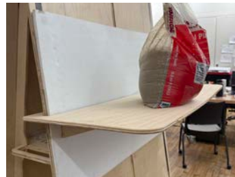
Adjustable platform designed to hold up to 50 lbs.
